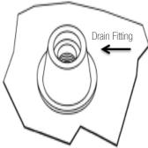
Step 1: Find the clear drain fitting located in the center of the unit. (It is likely that it will be in an inverted position)
